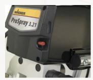
Maintenance is made easy with the Auto-Oiler\*. With the push of a button before each use the piston is oiled and the packings are lubricated. The "Easy Glide" machine oil can be refilled easily and forms a protective film around the cylinder and piston, protecting the unit against premature wear.
