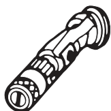
Tip marking Bore mm Spray width at about 30 cm removal of spray object Pressure 100 bar (10 MPa) Use Flat jet adjusting tip Order No. 15 0.13 - 0.46 5 - 35 cm Paints 0999 057 20 0.18 - 0.48 5 - 50 cm Paints, fillers 0999 053 28 0.28 - 0.66 8 - 55 cm Paints, dispersions 0999 054 41 0.43 - 0.88 10 - 60 cm Rust protection paints - dispersions 0999 055 49 0.53 - 1.37 10 - 40 cm Large-area coats 0999 056
