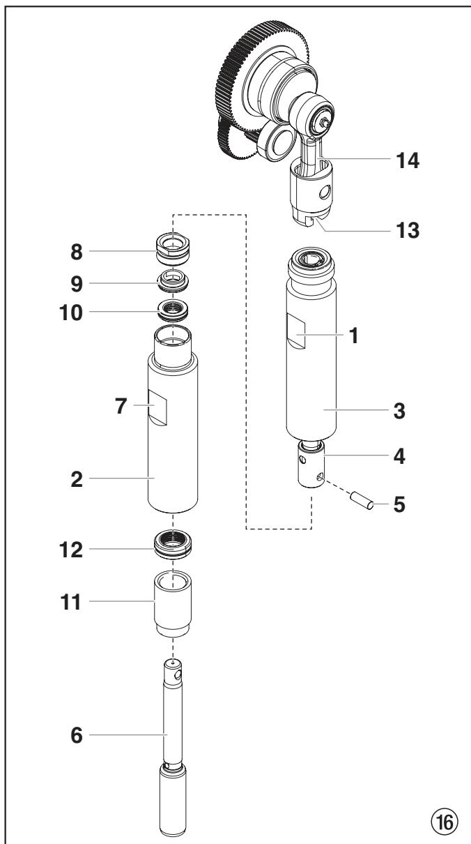
15. Clean the upper housing (2) and cylinder (3-5). Inspect the upper housing and cylinder for damage and replace if necessary.
