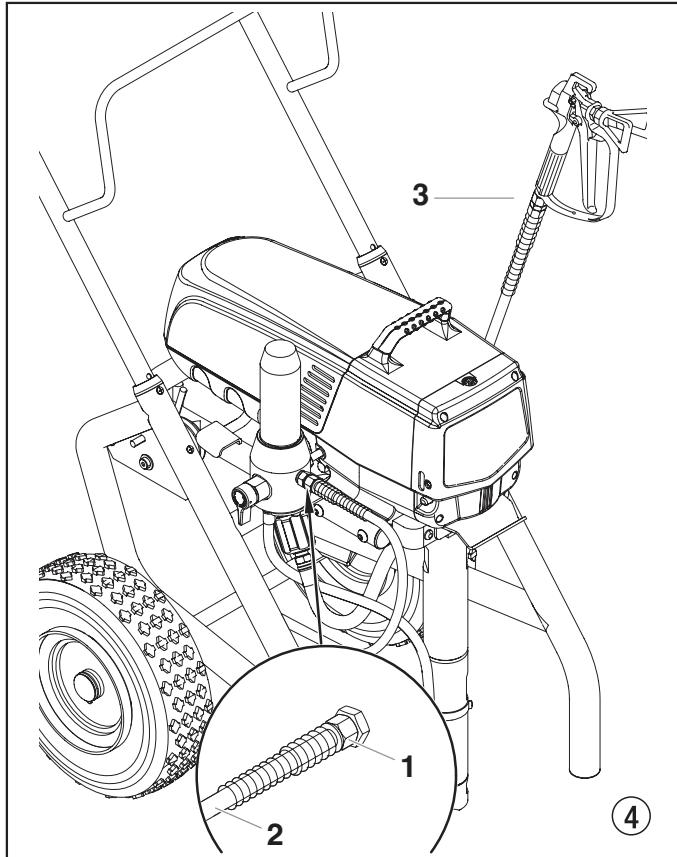
4. Remove the oil cup cap with a straight-slot screwdriver.
